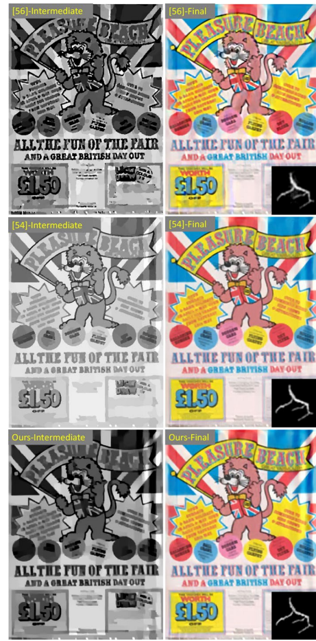
Fig. 34 Comparison of blind deblurring among state-of-the-art image priors in [54, 56] and our adaptive heavy-tailed priors. The kernel size is set as 65 \times 65
