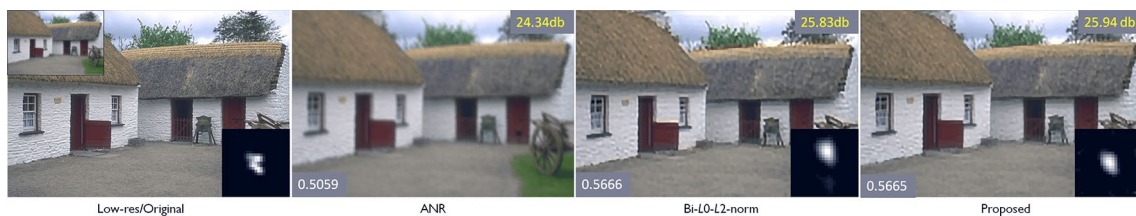
Fig. 16 Super-resolved images (3 times up-sampled) along with values of SSIM and PSNR by ANR [24] (0.5059, 24.34 dB), bi- L_0 - L_2 -norm [50] (0.5666, 25.83 dB) and our approach (0.5665, 25.94 dB)
