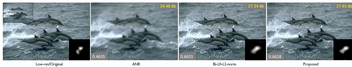
Fig. 13 Super-resolved images (3 times up-sampled) along with values of SSIM and PSNR by ANR [24] (0.4635, 24.48 dB), bi- L_0 - L_2 -norm [50] (0.6631, 27.34 dB) and our approach (0.6628, 27.45 dB)
