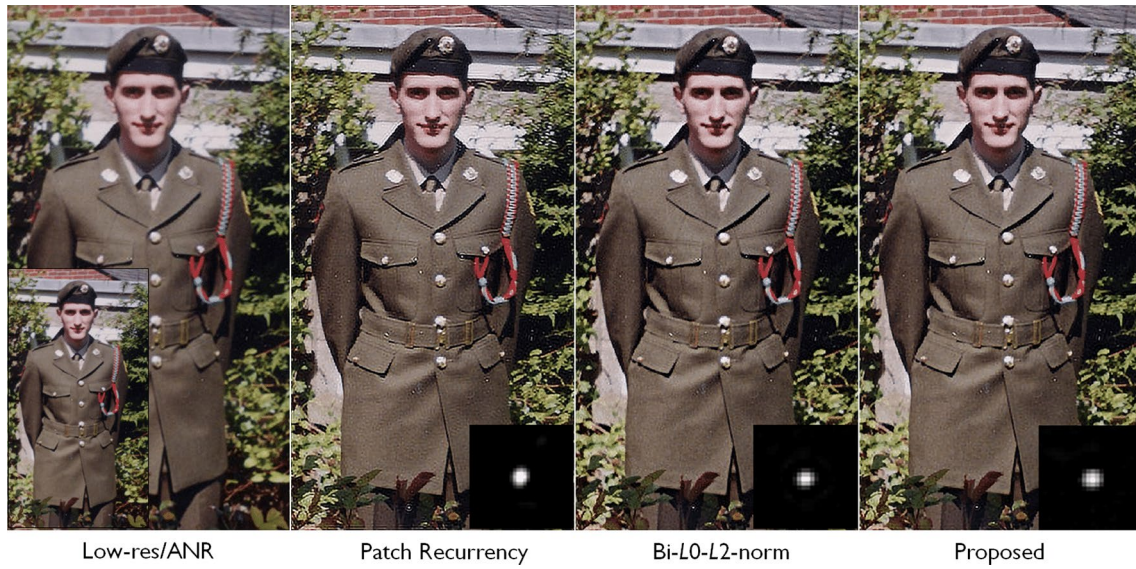
Fig. 19 Blind super-resolution (2 times) by ANR [24], Patch Recurrency [48], bi-L_0-L_2 -norm [50] and the proposed approach
